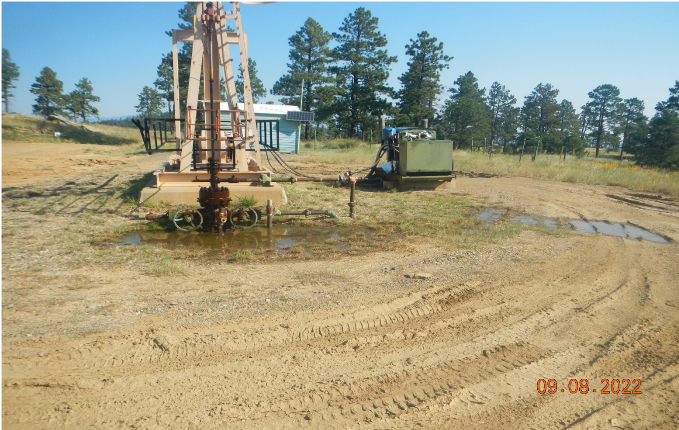
Photo 2. There is a water leak coming from the wellhead that needs to be repaired.
