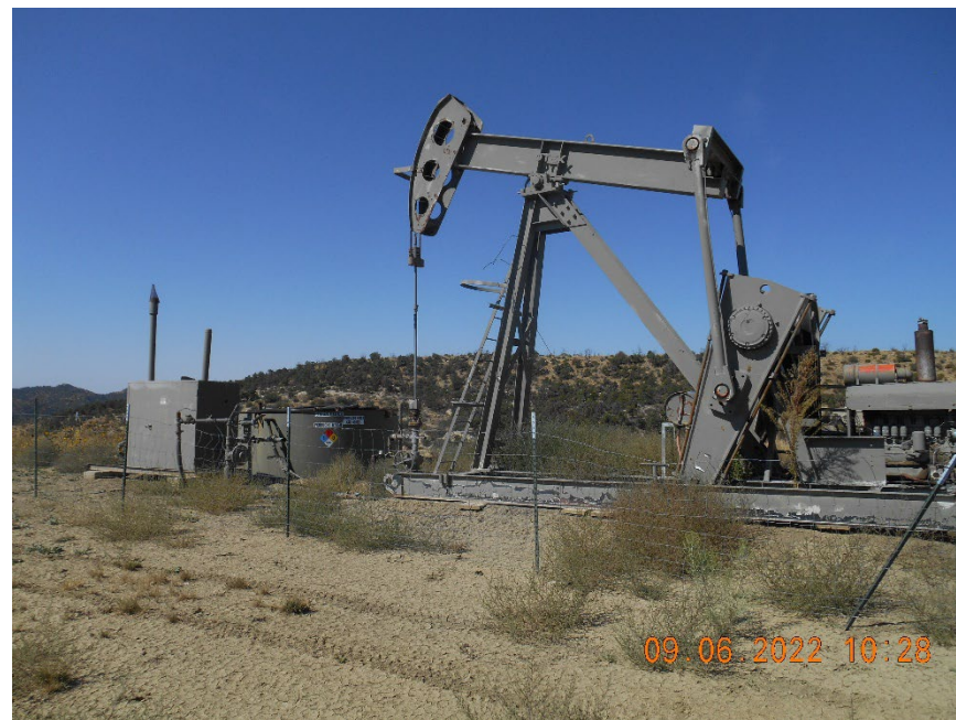
Wellhead with Pump Jack, Separator and Produced water tank
