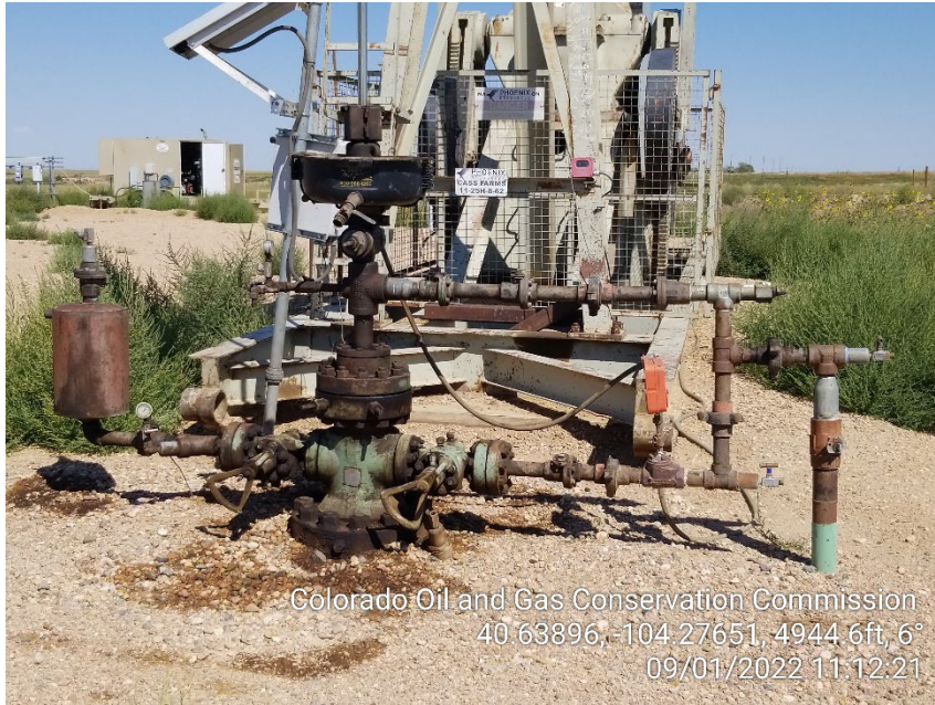
Photo 5 – Wellhead – Stained Soil
