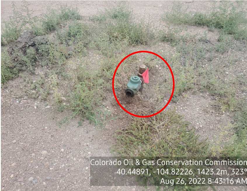
Photo 7: Marked riser to be removed
