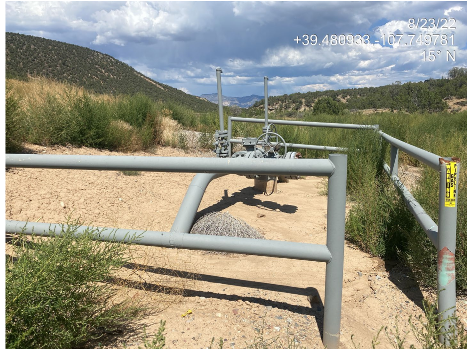
Photo 2. Photo taken from the southeast of the Location shows a pig launcher/receiver remaining on Location.
