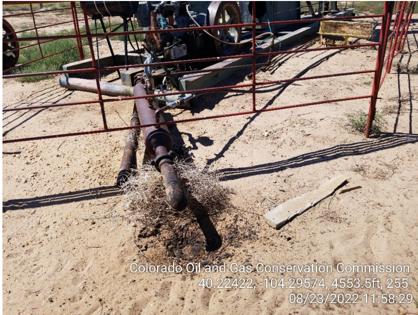
Photo 3 – Stained Soil at Exhaust
