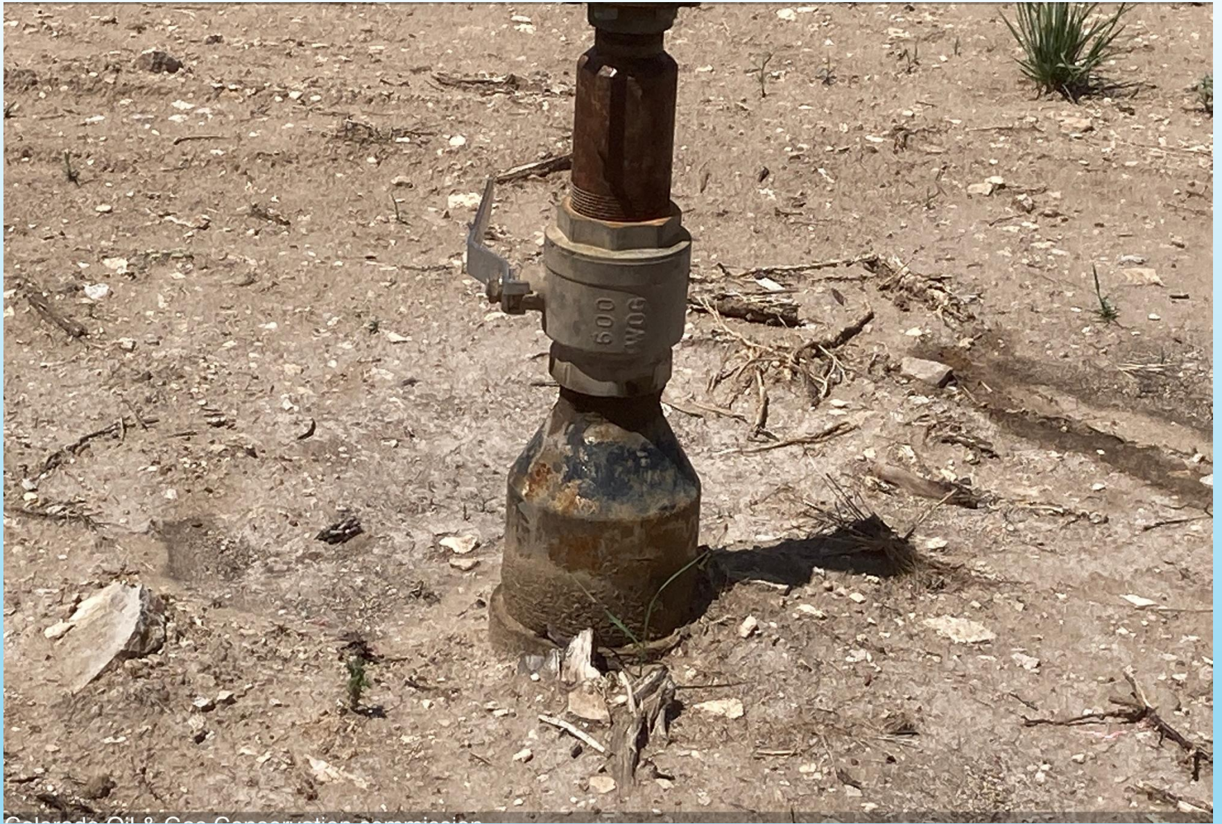
PHOTO 3: Bradenhead inaccessible or not visible. Install appropriate fittings to allow bradenhead visual inspection as per Rule 419.a.(1), (2). CA DATE 8-30-2022.
