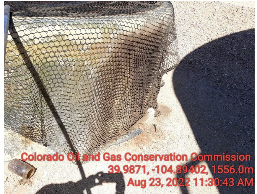
Photo 8 stained soil around Produced water tank.
