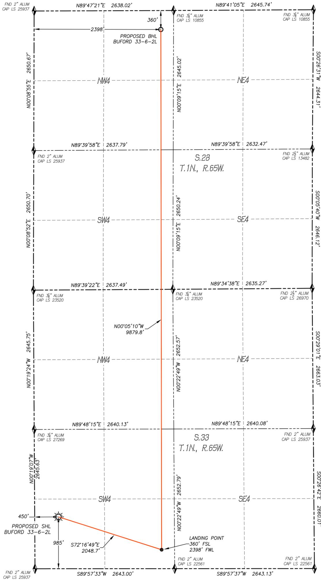
IN ACCORDANCE WITH A REQUEST FROM CONFLUENCE RESOURCES, DALEY LAND SURVEYING, INC. HAS DETERMINED THE SURFACE LOCATION OF THE BUFORD 33-6-2L WELL TO BE 985' FSL, 450' FWL, AS MEASURED AT NINETY (90) DEGREES FROM THE SECTION LINES OF SECTION 33, TOWNSHIP 1 NORTH, RANGE 65 WEST AND THE BOTTOM HOLE LOCATION TO BE 360' FNL, 2398' FWL, AS MEASURED AT NINETY (90) DEGREES FROM THE SECTION LINES OF SECTION 28, TOWNSHIP 1 NORTH, RANGE 65 WEST, OF THE 6TH PRINCIPAL MERIDIAN, WELD COUNTY, COLORADO.
