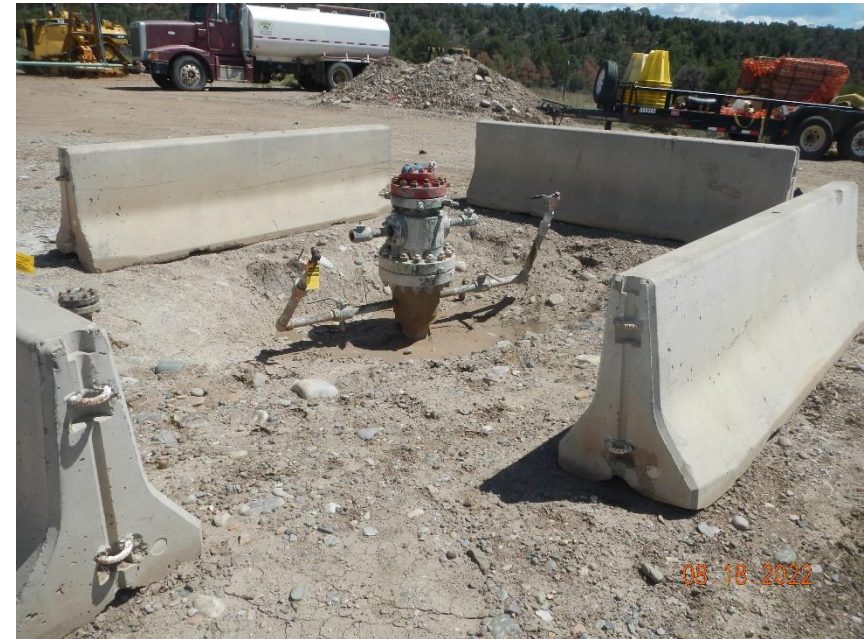
Hott 20-2 1 well not cut and capped
