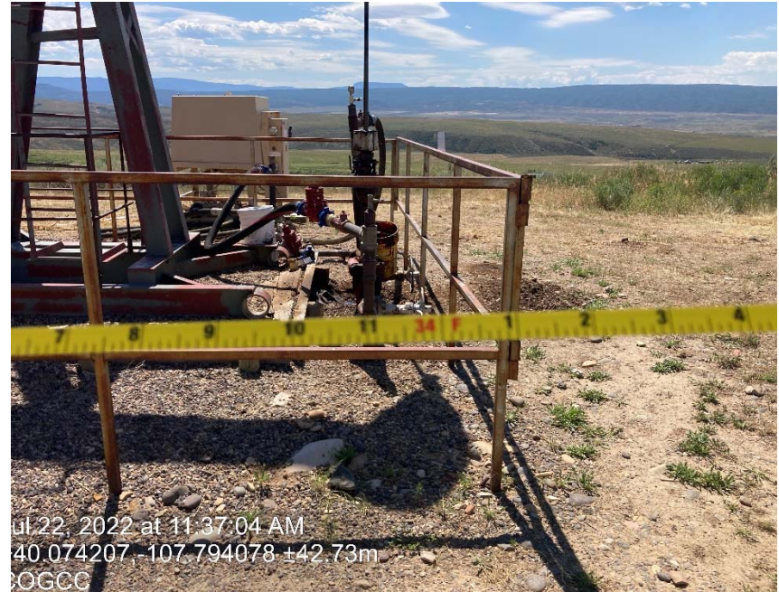
Tape measure from closest generator from well head. Approx. 34 feet away from well head.
