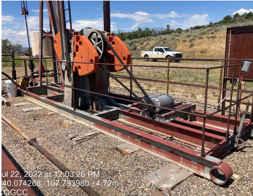
Pump jack belts missing guard
