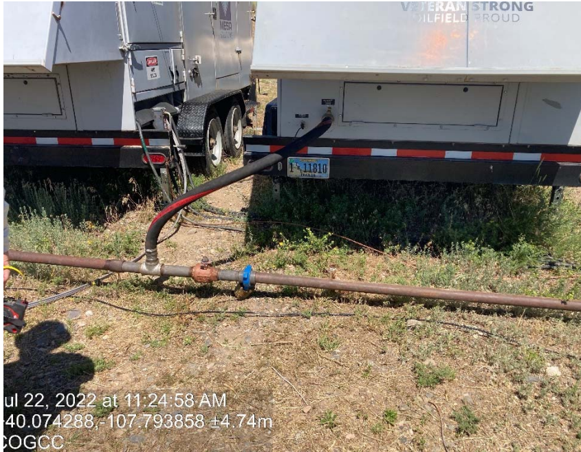
Line from well head connected to generator
