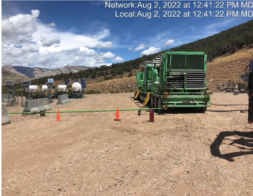
Photo #7381 Portable compressor being used to unload the PE25 federal 25-5A well.
