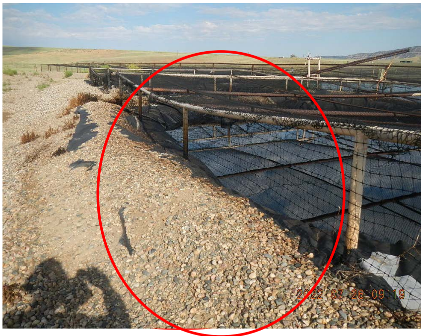
Oil on top of berm of first pit.
