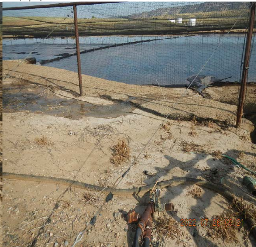
Fluids flowing from transfer pump. Reportable Spill/Release. Operator was notified verbally on 7/26/2022 and via email on 7/27/2022. Note sediment debris fan into pit.
