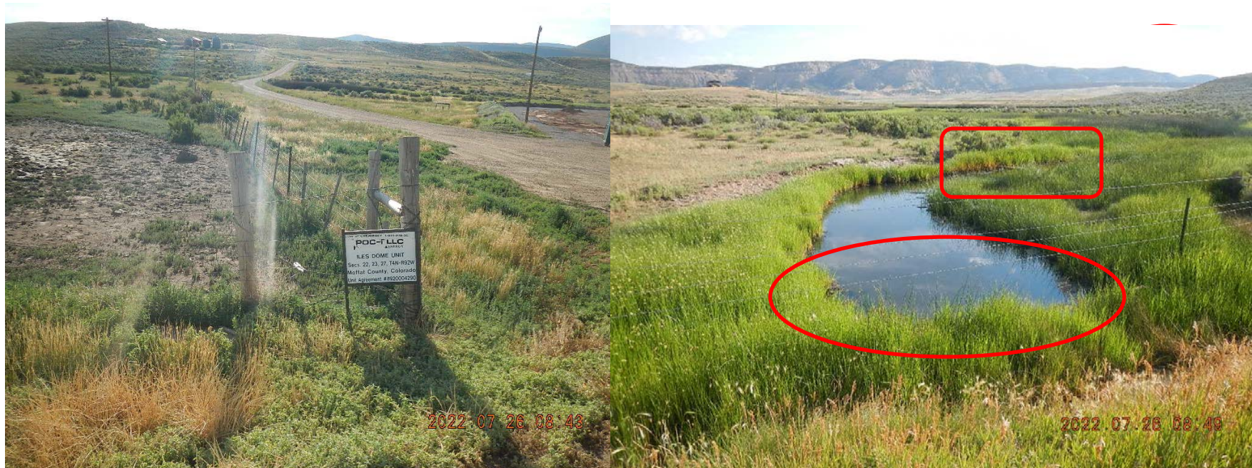
Outfall of culvert beneath County Road LY5. Oily impacted vegetation and oil on the water surface. Booms are placed down gradient.
