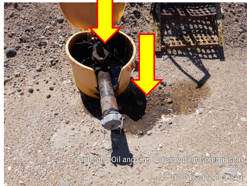
Photo 6 – Oily Waste and Stained Soil at Loadline Bucket
