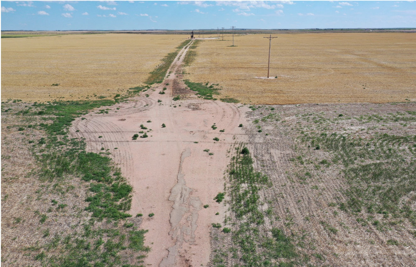
Photo 1. Drone aerial photo facing south toward the location. The access road travels thru the location to an active well site. The area out side of the road at the disturbed location has not been reclaimed. Previous corrective action was not completed.
