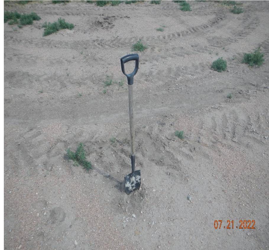
Photo 7. The soils throughout areas of the location are compacted. The shovel could not penetrate through the soil surface.
