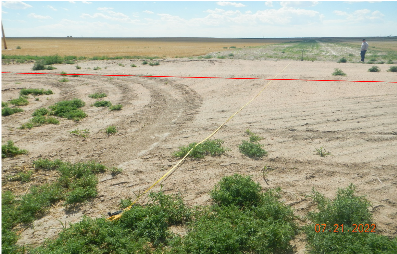
Photo 4. Facing west toward the location which remains with no crop growth. A 100 ft. tape measure shows the length of disturbance. The road travel thru the center location at the red line. There is approximately 50 ft. of disturbance with no crop growth at the west and east side of the access road.
