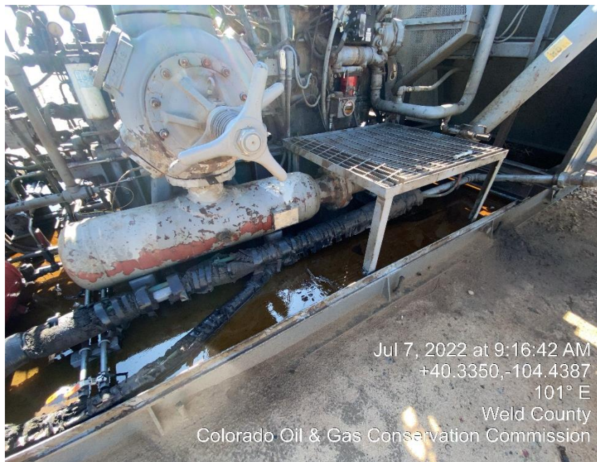
Photo #7 Oily Waste on Compressor skid & Mechanical Conditions
