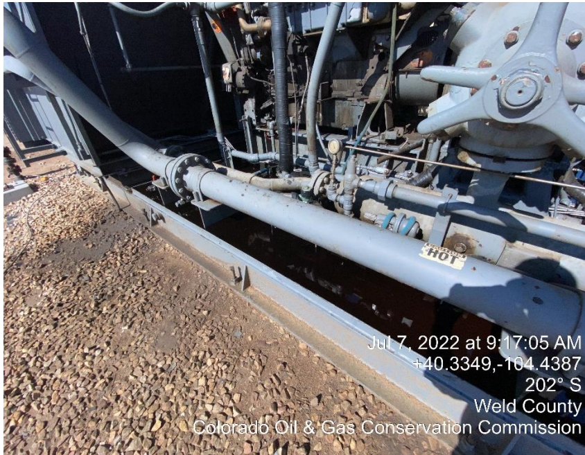
Photo #3 Stained Soil & oily waste on compressor skid
