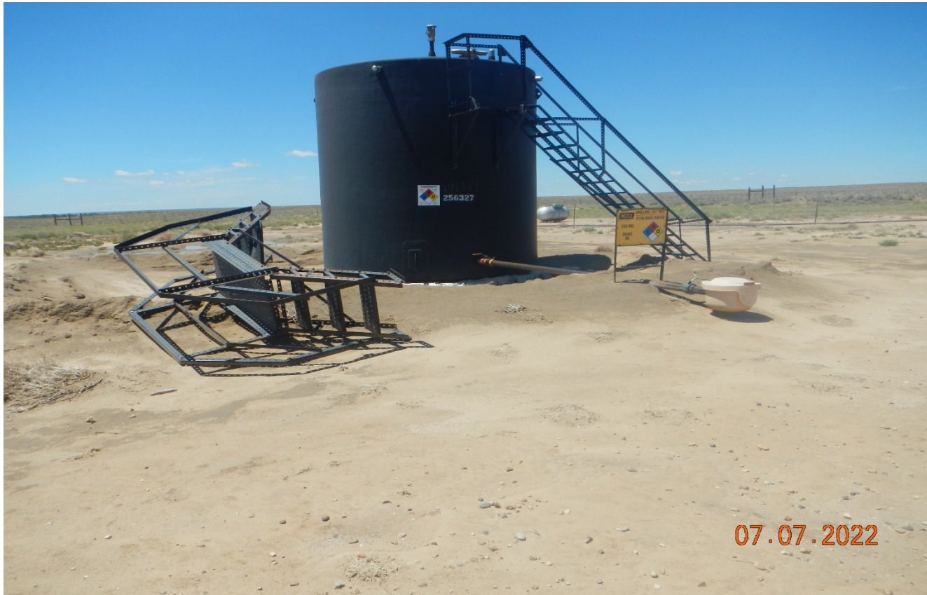
Photo 7. Facing southeast toward the location. The catwalk is tipped over and not in use and should be removed.
