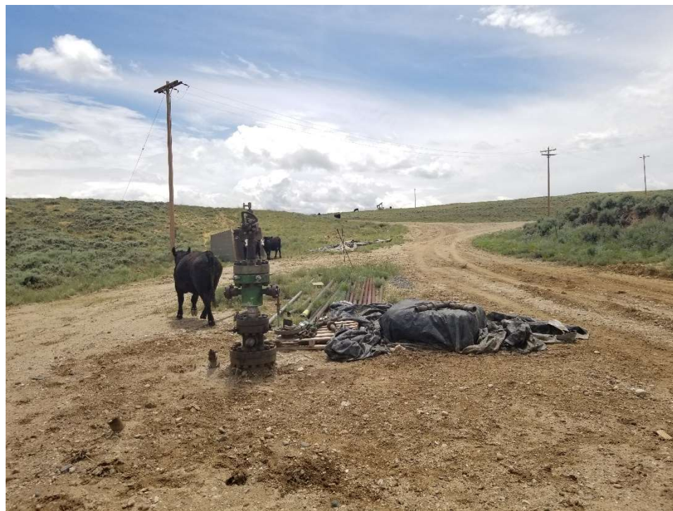
Photo 1. Overview of location taken facing south. No wellhead sign. Debris/equipment on location.
