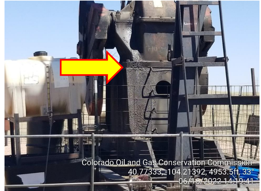
Photo 6 – Gear Box Leak
