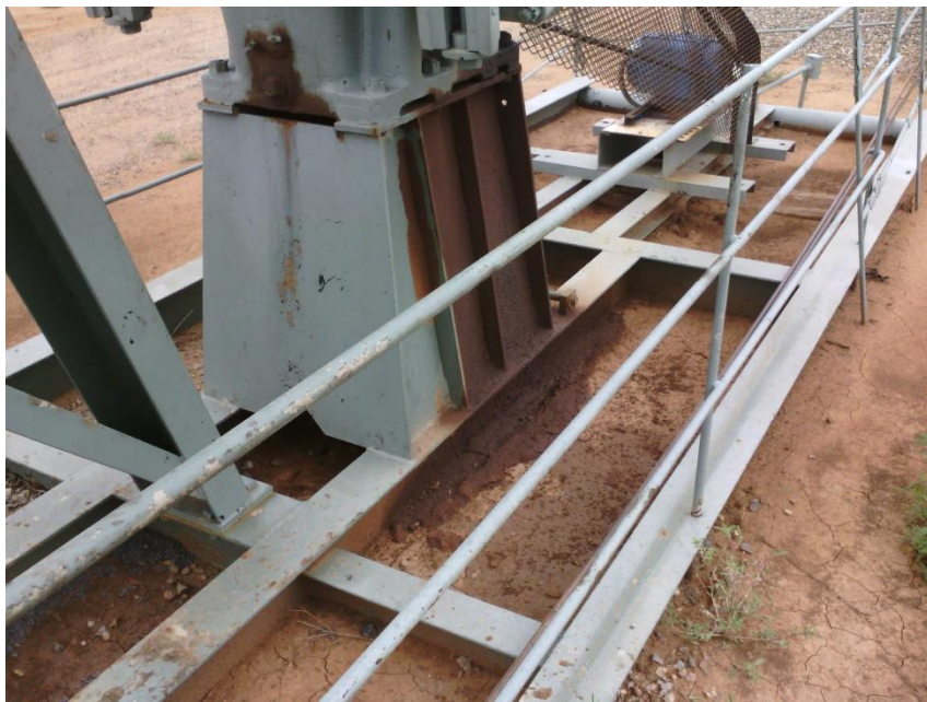
Gear box leak and impacted material
