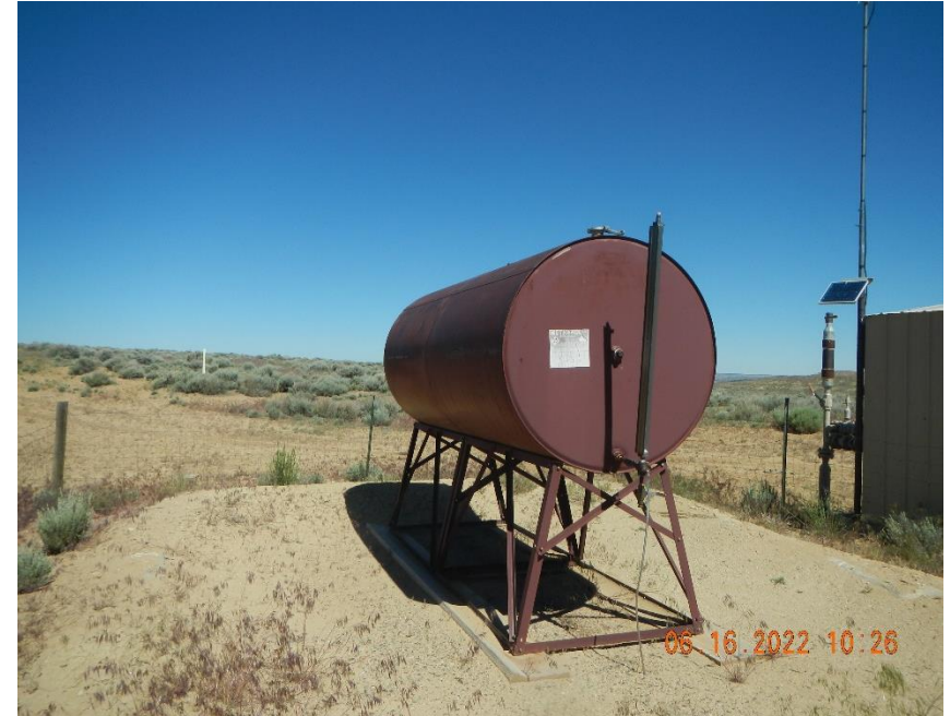
Metal tank by meter shed and separator NFPA, contents, and capacity are faded.
