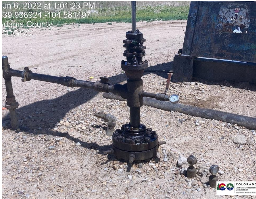
Pic 3 mechanical issue with wellhead, oil is covering wellhead
