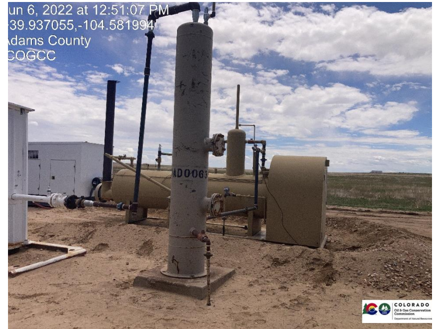
Pic 7 Vertical separator, horizontal separator
