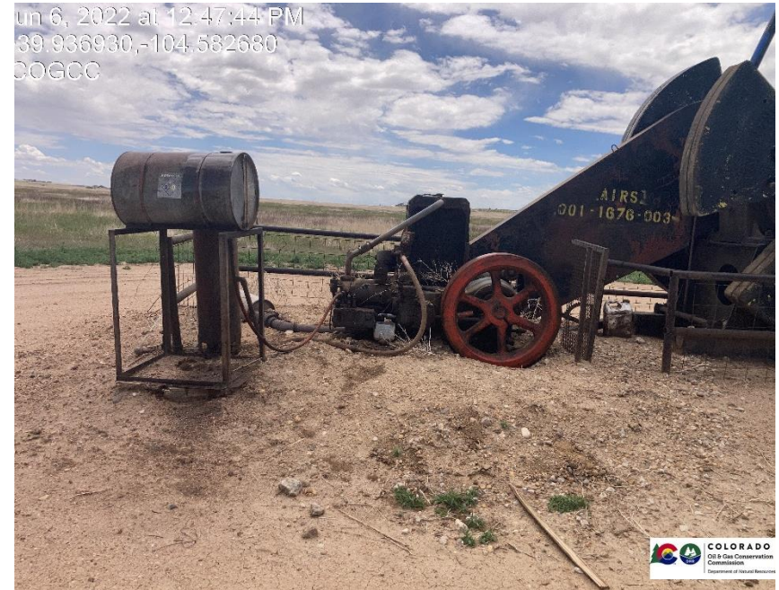
Pic 2 stained soil, mechanical issue with gas motor, trash on location, no BMP under chemical tanks
