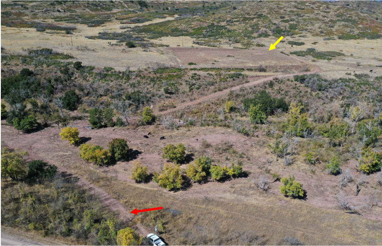
Photo 1. Drone aerial photo facing northwest toward the access road and the location. Red arrow points the the access road and yellow arrow points to the location which have not been reclaimed per rule 1004. Photo taken on 10/5/2021
