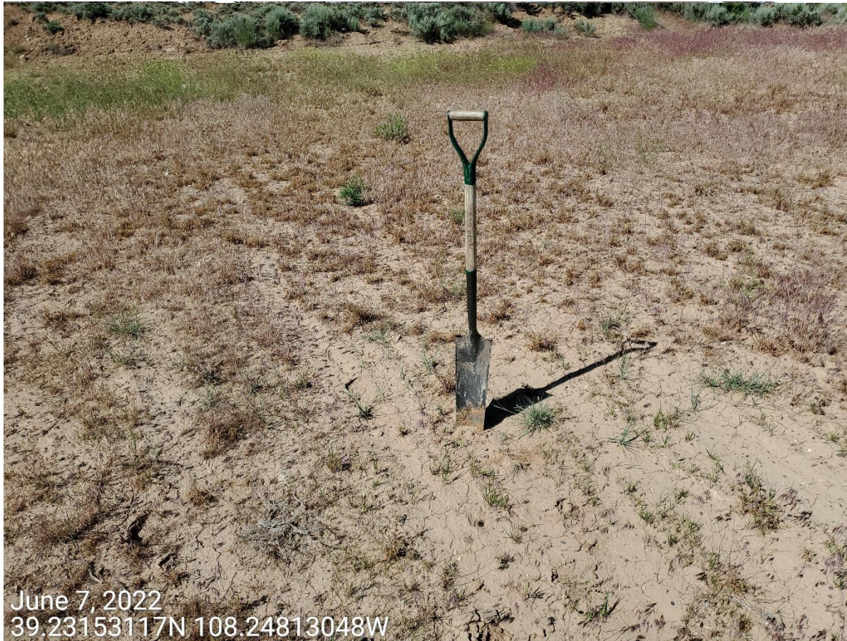
Photo 3: Photo shows compaction issues are evident; Location has not been decompacted.
