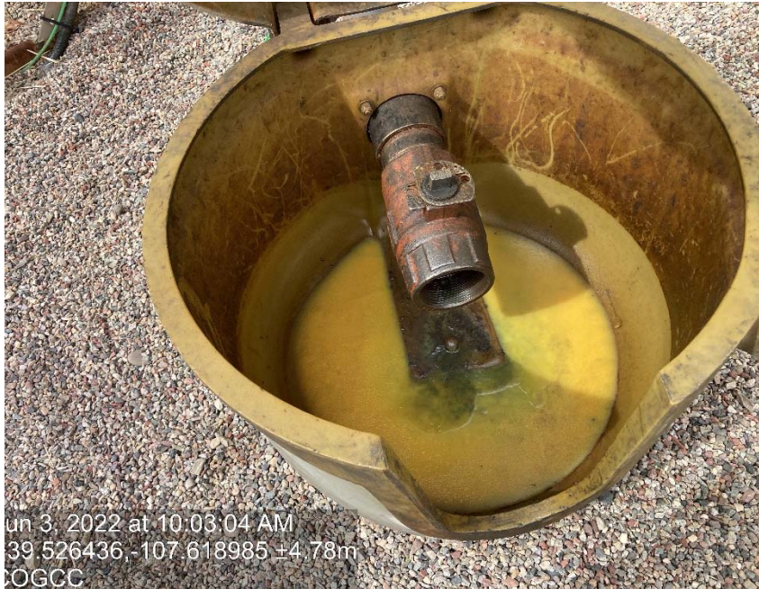
Valves missing cap/plug
