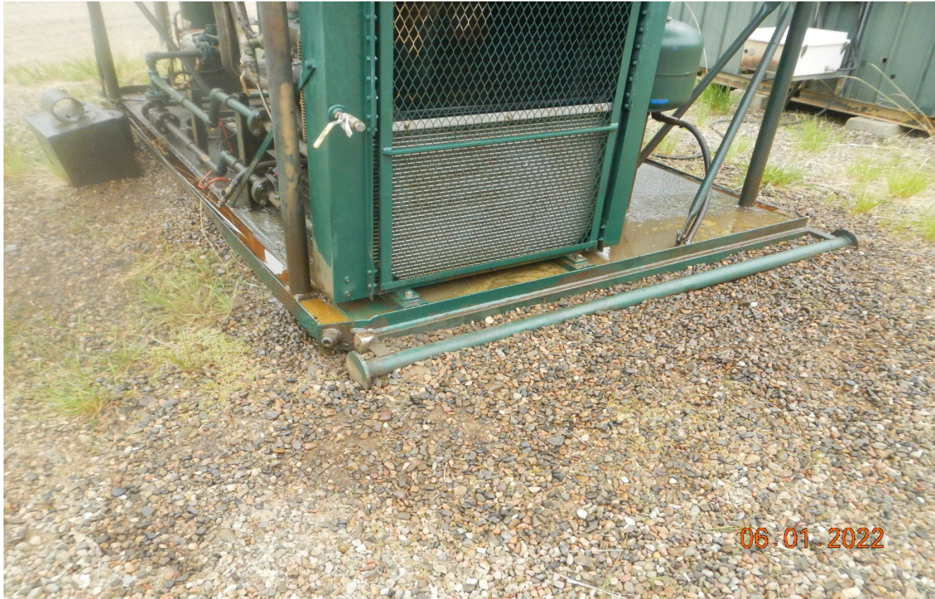
Photo 2. There is oil I the engine skid that has spilled over that needs to be cleaned up.
