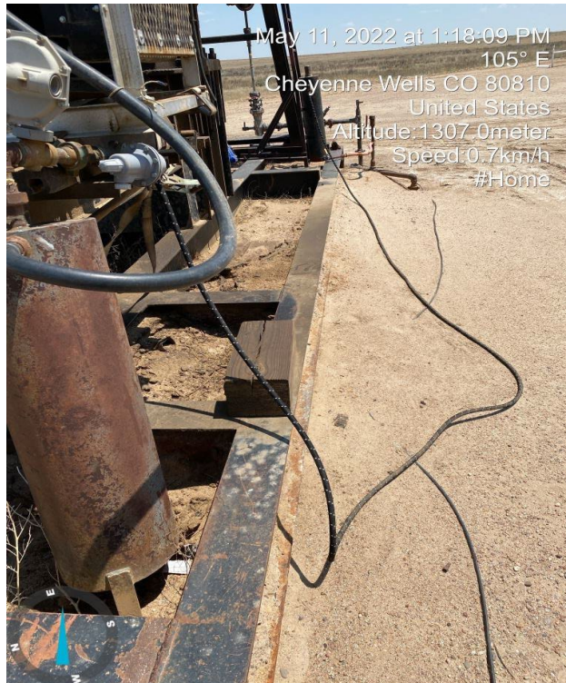
7. Gas supply line from wellhead scrubber to engine scrubber.
