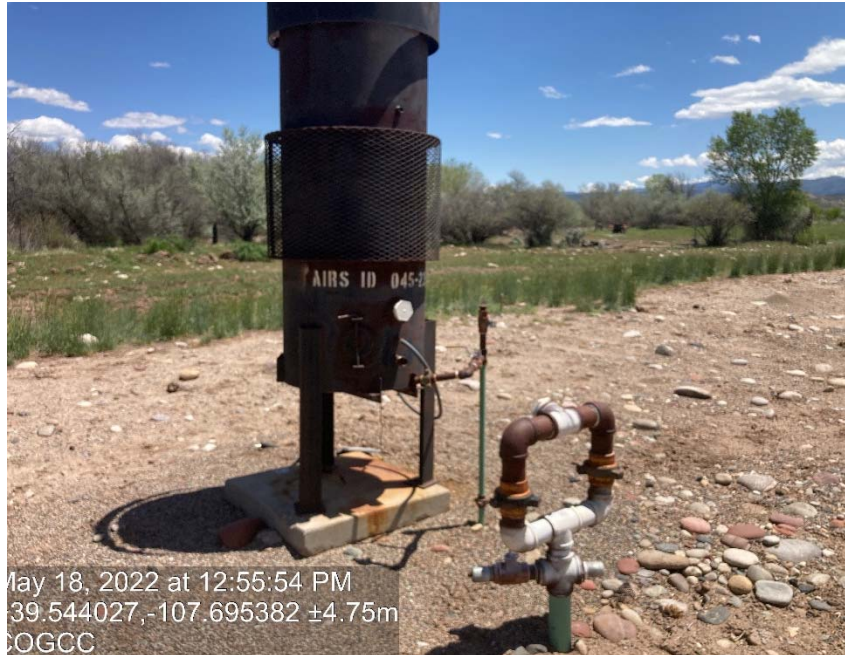
ECD disconnected (stored equipment) not anchored
