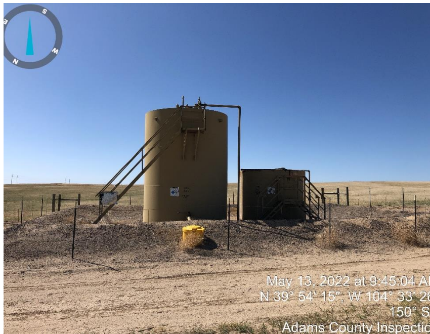
Photo #1 Crude tank and produced water tank.
