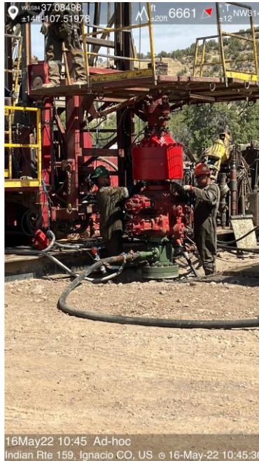
IMG 11 Wellhead with BOP
