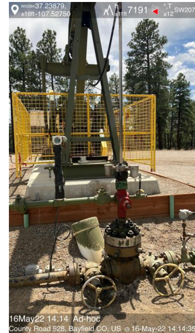
IMG 16 Pump jack and wellhead
