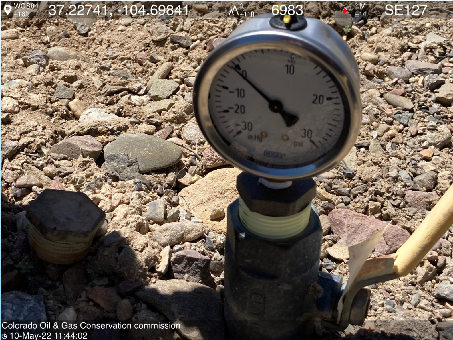
PHOTO 6: BRADENHEAD PSI 0. MONITORED FOR 15 MIN. NO BLOW NO FLOW.
