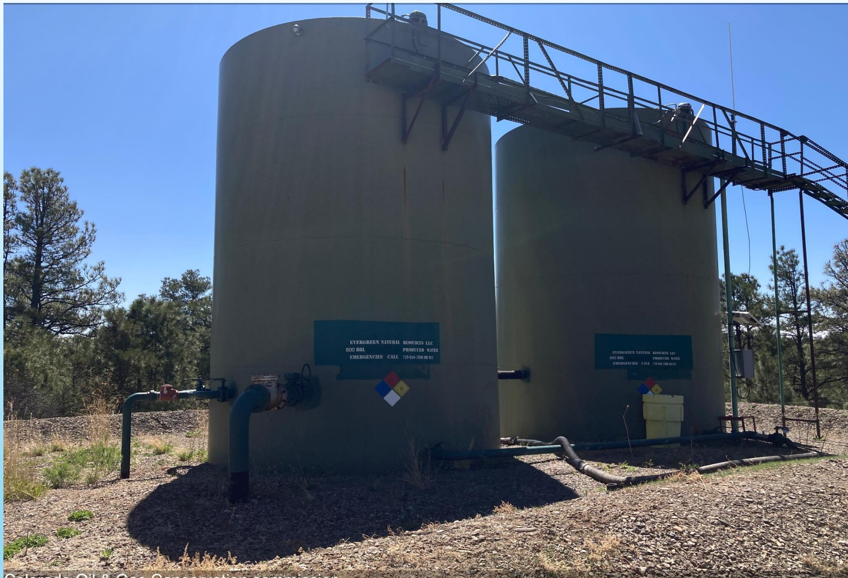
PHOTO 3: TANK BATTERY
