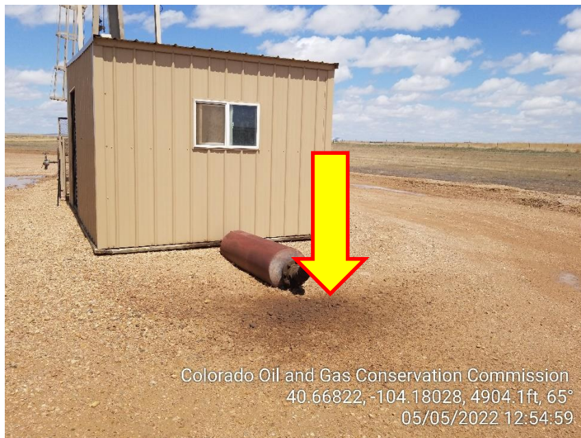
Photo 3 – Stained Soil at Exhaust
