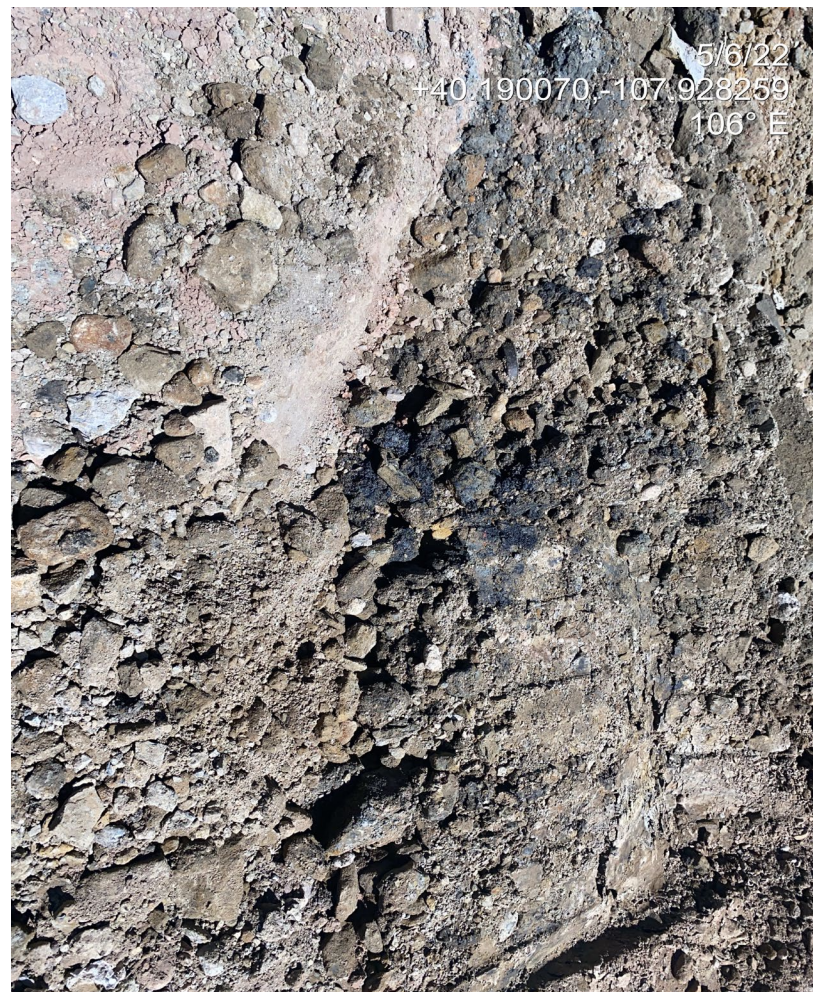
Photo 4. Photo taken from the area of the excavated well shows stained soils around the well. A strong hydrocarbon odor was present at the time of this inspection.
