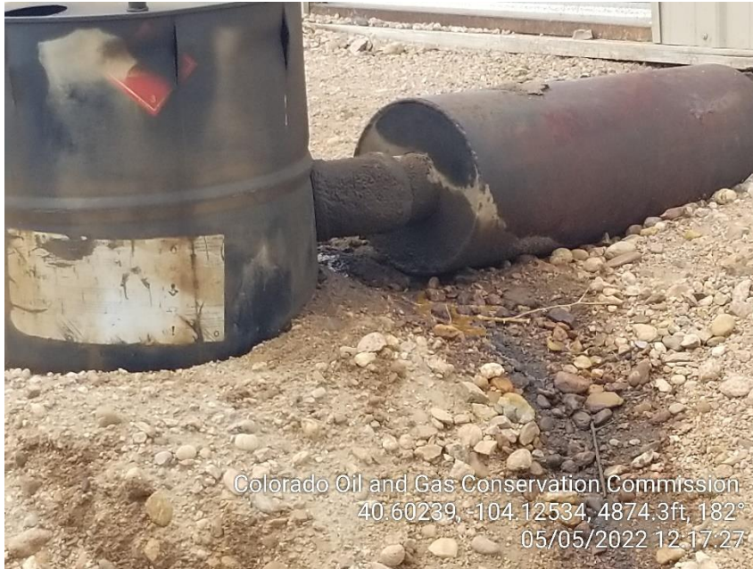
Photo 7 – Stained Soil at Exhaust
