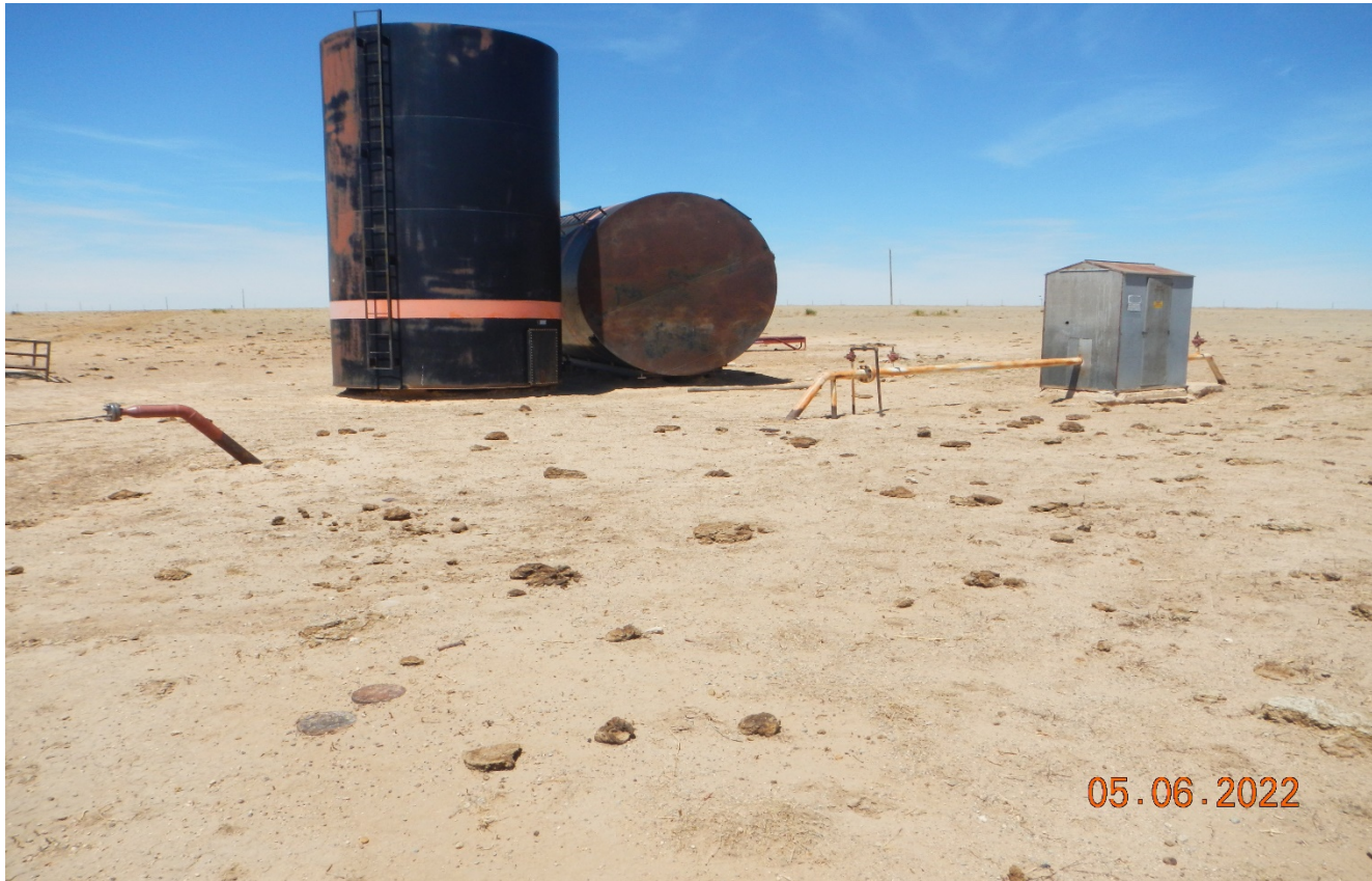
Photo 4. There are two tanks, pipe riser, and meter run that remain. All equipment should have been removed within 3 months of well abandonment.
