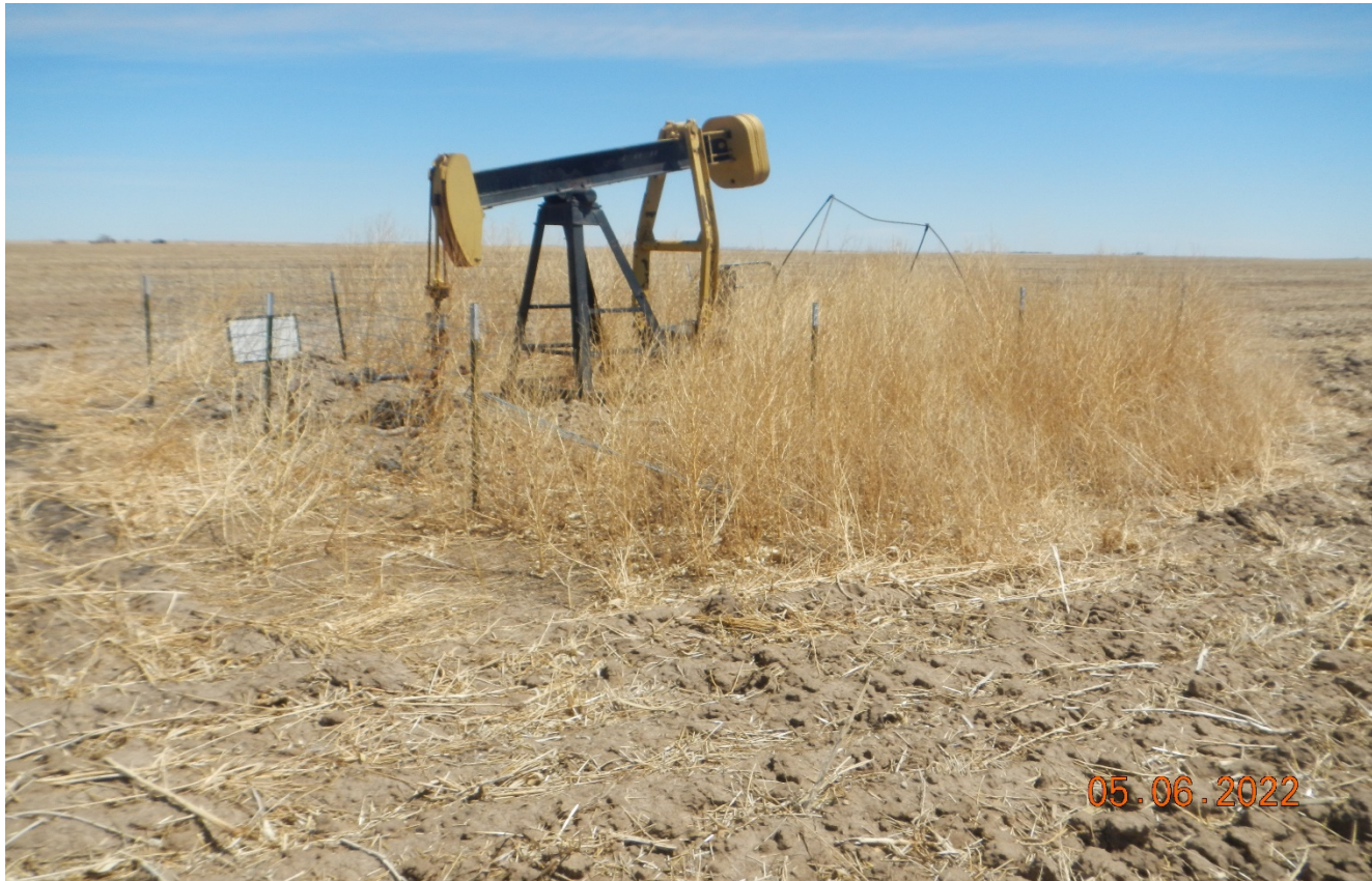
Photo 2. Facing toward the well site. There is weed debris near the pumpjack which is a fire hazard.
