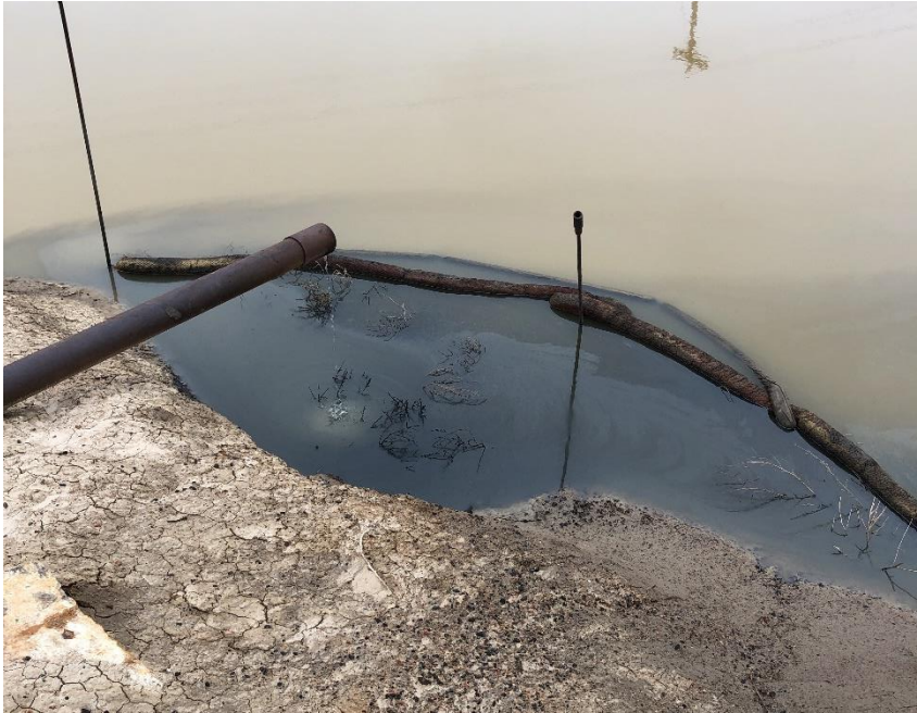
Photo #9 Hydrocarbons present in produced water pit.
