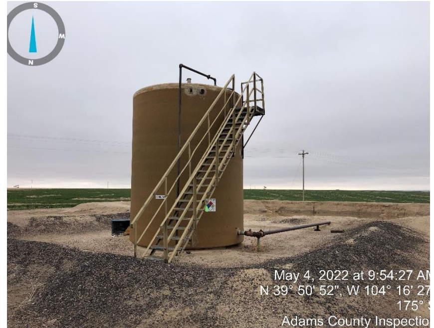
Photo #6 produced water tank.
