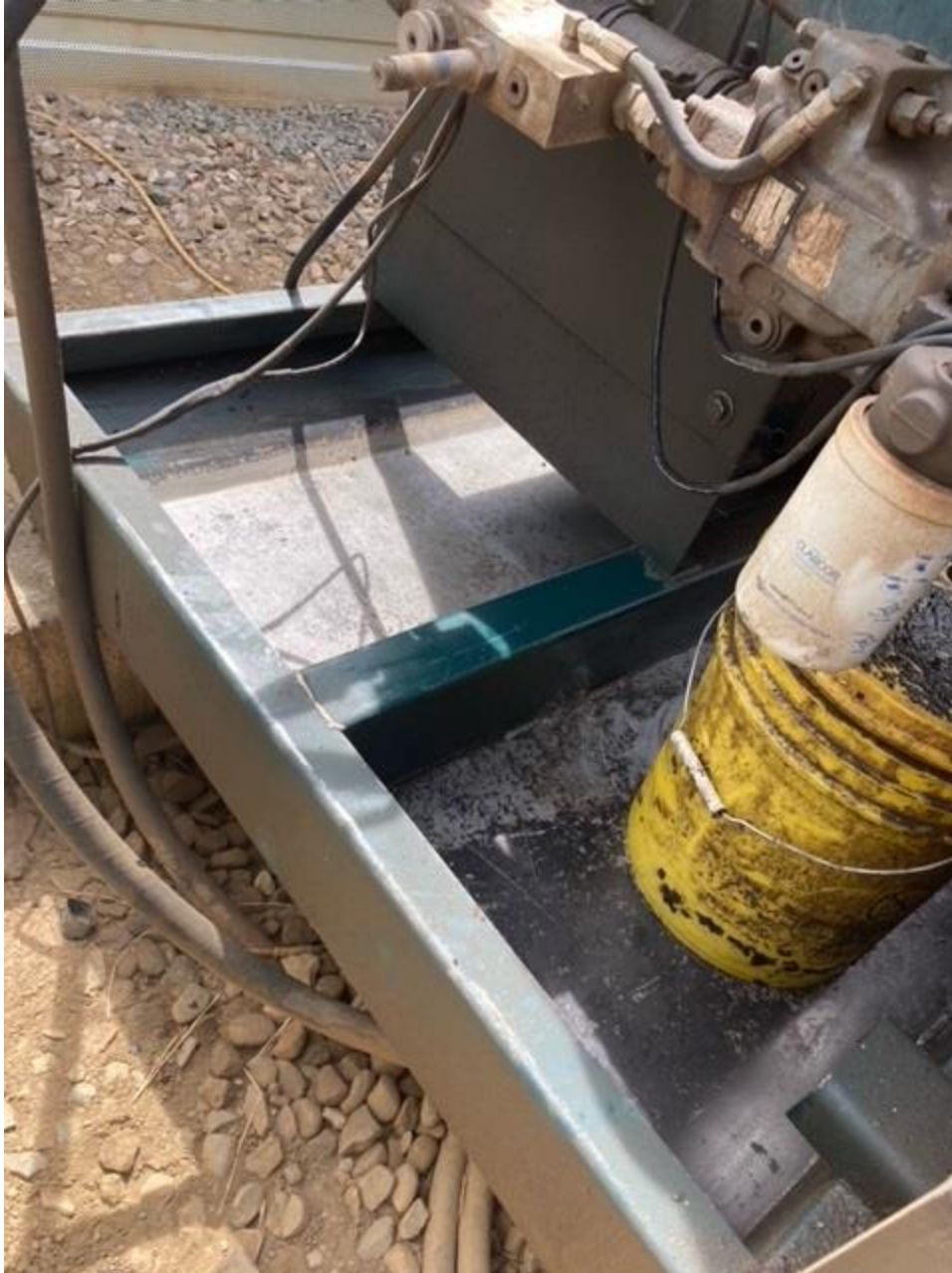
Complied with Rule 1002.f.(2)B, Complied with general provisions of the oil and gas act for wildlife protection and SB-181. (Tightened flange on pump that had very small hydraulic leak.)
