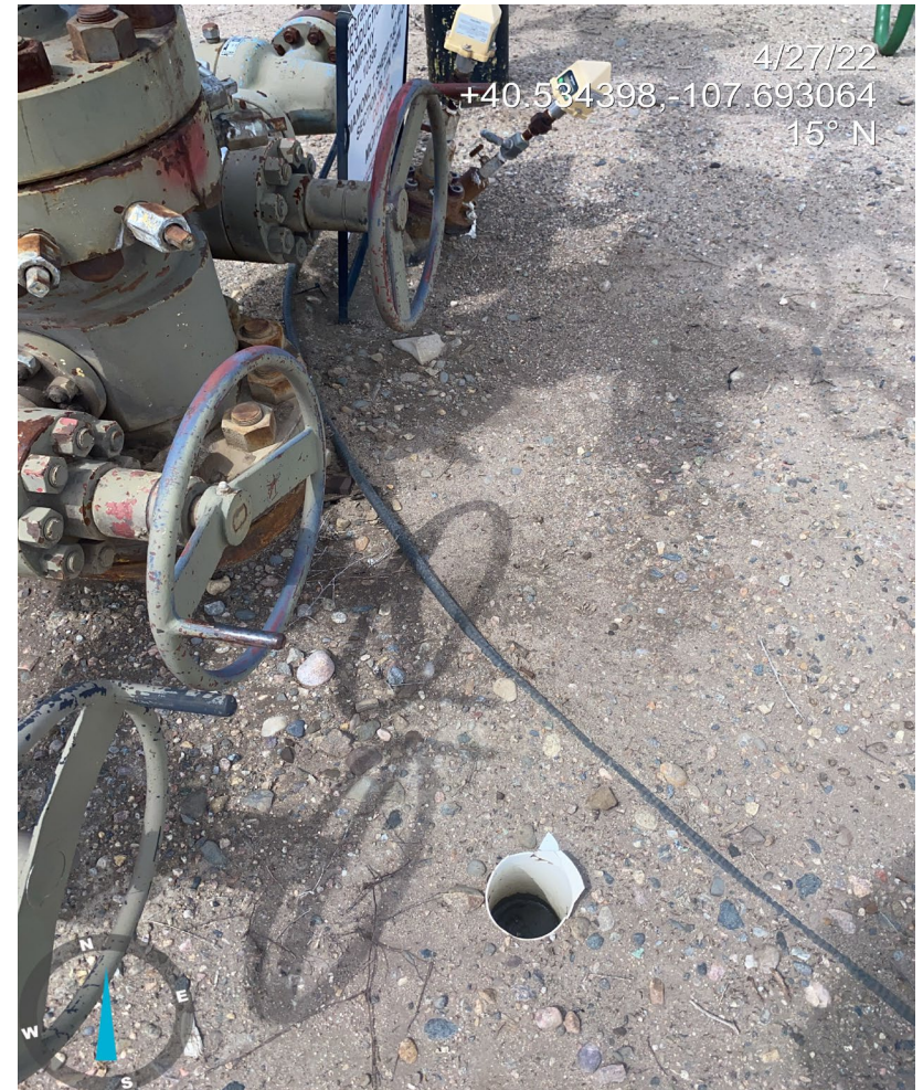
Photo 30. Photo shows an open pipe at well API # 05-081-07804.
