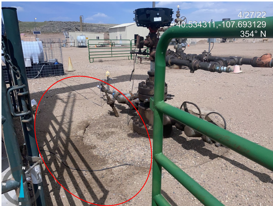
Photo 29. Photo shows stained soils around well API # 05-081-07817
