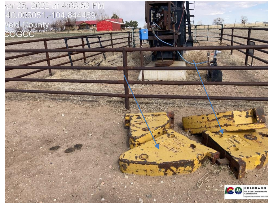
Pic 6 unused counterweights for pump jack need to be removed from location
