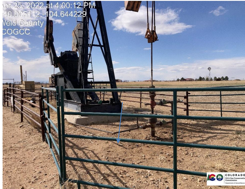
Pic 1 wellhead, arrow points to bradenhead
