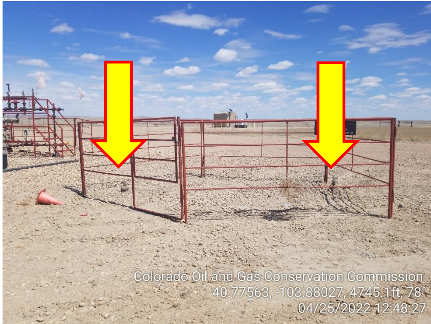
Photo 3 – LD06-620 Wellhead – PA – Cut and Capped. Unmarked Risers
