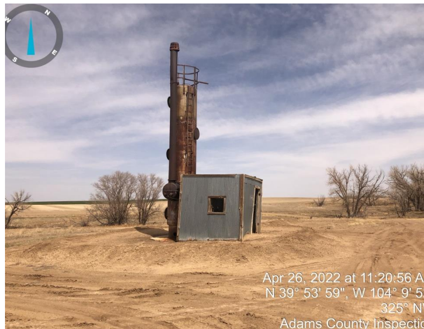
Photo#2 Vertical Separator
