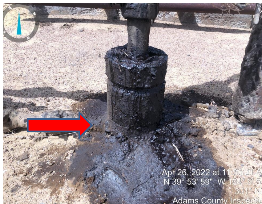
Photo#16 Wellhead leaking
