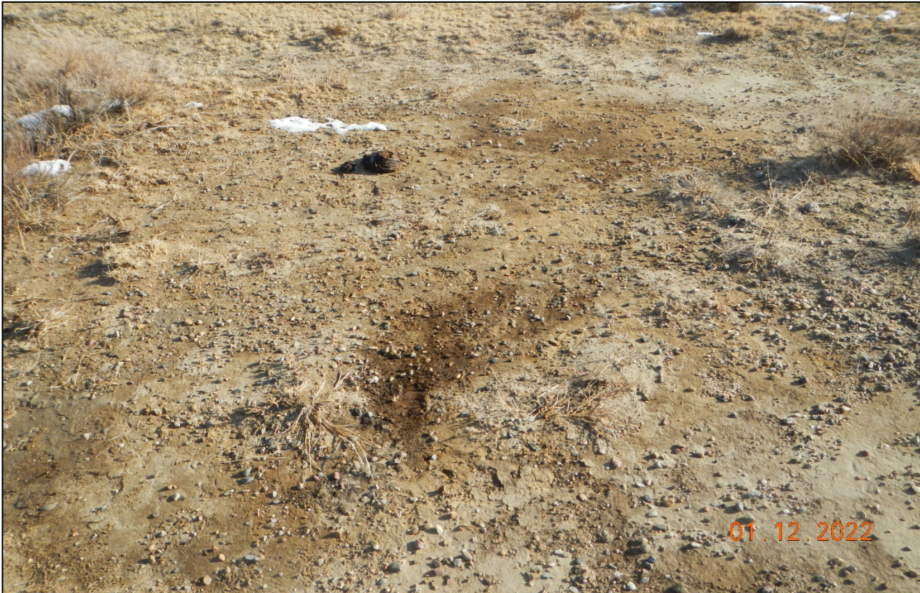
Photo 3. Ground cover at center of the location. There is darkened soils in this area with a hydrocarbon odor. Contaminated soils need to be properly removed and disposed.
