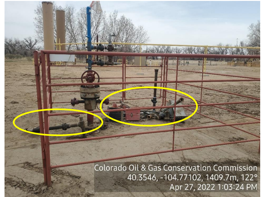
Photo 2: Wellhead. Disconnected equipment
