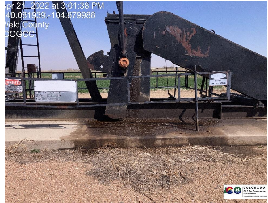
Pic 2 leaking gear oil/stained soil/mechanical issue.
