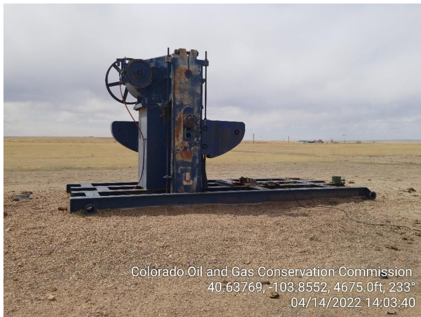
Photo 5 – Sub Base, Gear Box and Counter Weights
