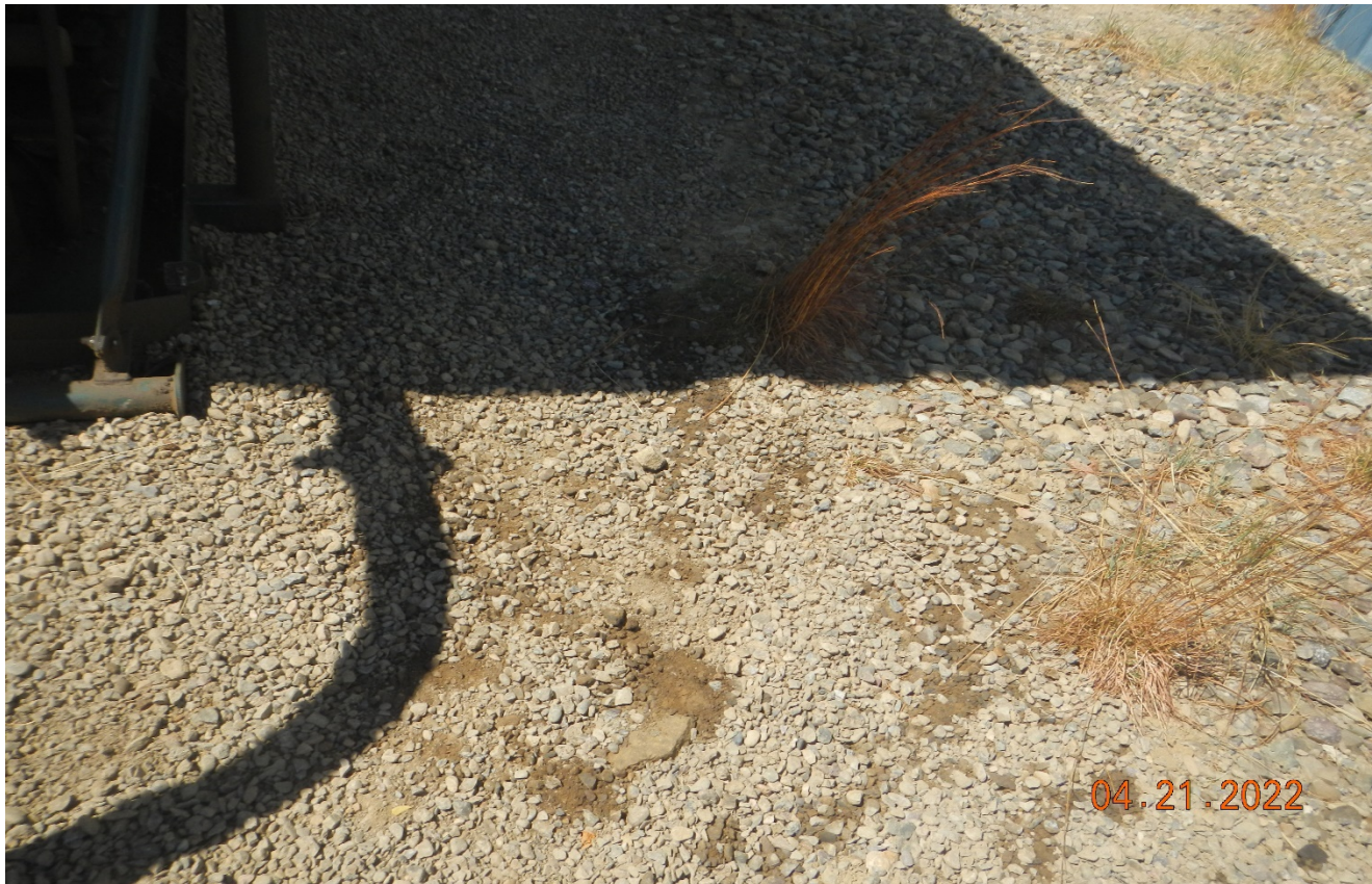
Photo 3. There is stained soils visible underneath the gravel.
