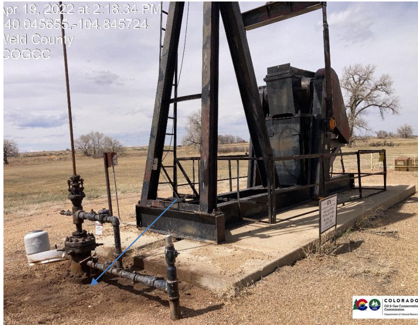
Pic 1 stained soil near wellhead/mechanical issue.
